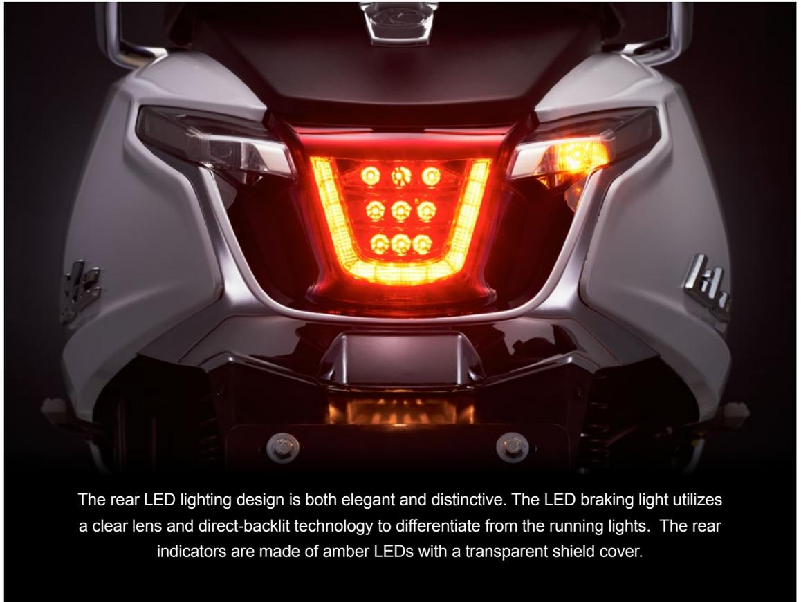
The rear LED lighting design is both elegant and distinctive. The LED braking light utilizes a clear lens and direct-backlit technology to differentiate from the running lights. The rear indicators are made of amber LEDs with a transparent shield cover.
